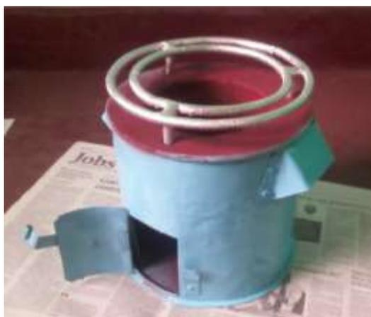
**Thermal efficiency: 26%.** The manufacturer's information on efficiency of the cook stove is substantiated by results of the testing performed at University of Nairobi, Kenya. The cook stove has been tested according to the Water Boiling Test protocol.
